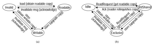
Figure 1: Idealized protocol state machine for (a) the non-home side, and (b) the home side. Transitions are labeled with causes and, in parentheses, actions.
