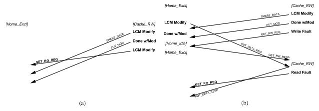
Figure 6: Two different scenarios in which a GET\_RO\_REQ arrives in state Home\_Exclusive. The appropriate response to the message is different in each case.
