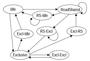
Figure 2: State machine (home side) with intermediate states necessary to avoid synchronous communication.
